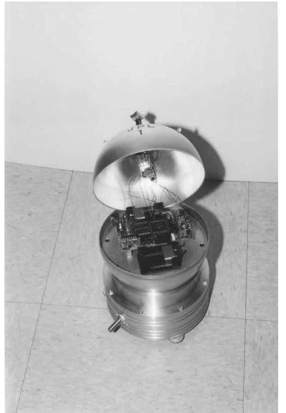
Fig. 3 Photograph of the interior of the model spacecraft showing the miniboard micro-controller, sensor unit, batteries, and the interface electronics.
